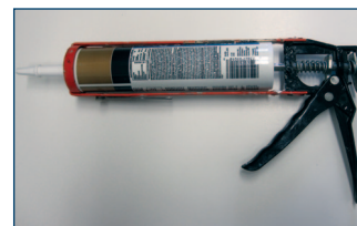
Figure 5. Caulking gun and sealant.
