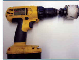
Figure 8. Drill and 2 3/8-inch hole saw.
